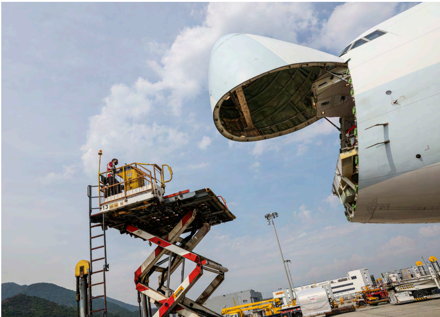
Nose loading, a benefit of the 747-8F. Photo courtesy Cathay Pacific.
